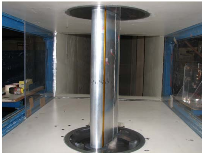
Figure 3. A picture of the airfoil in the wind tunnel.
